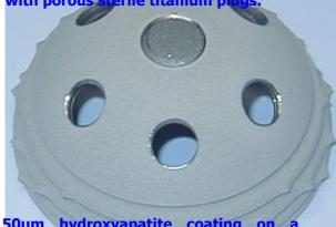
150µm hydroxyapatite coating on a 20µm porous titanium sub-layer surface.
